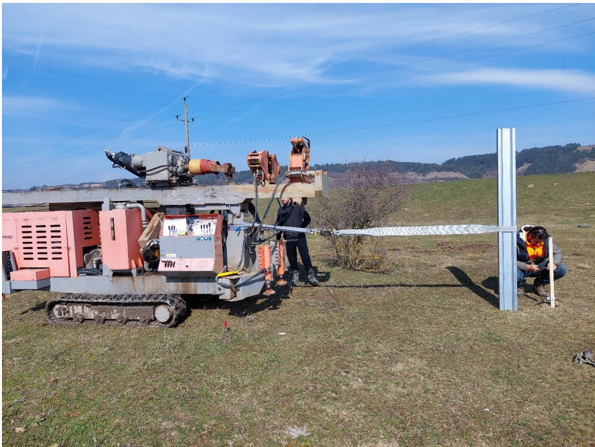
Fig. 9. Titan Pride 120 drilling rig tied to a Sigma metallic profile
