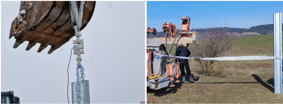
Fig. 7. The force sensor coupled vertically (left) and horizontally (right)
